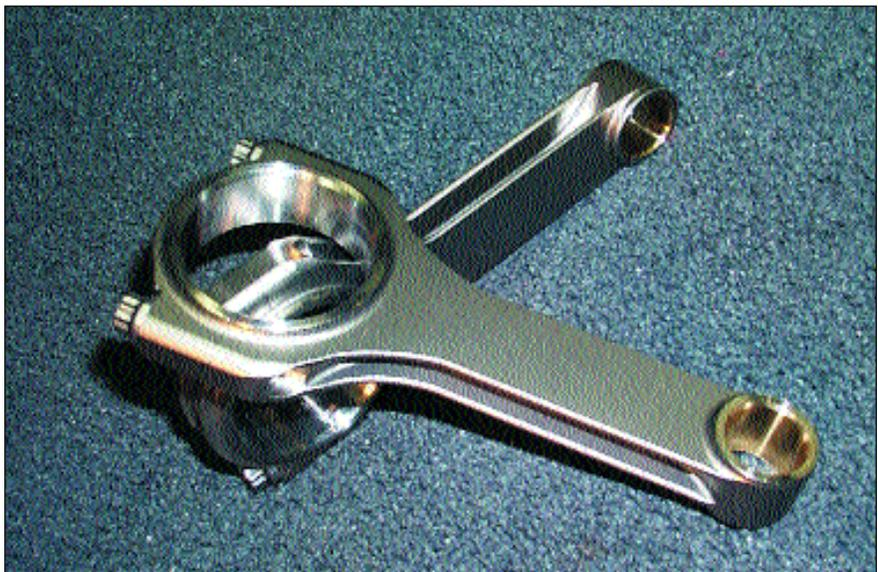
*Connecting rods usually fail in fatigue. These lightweight, forged 300M steel connecting rods use cryogenic processing to resist the forces generated by an engine turning over 9000 rpm.*
